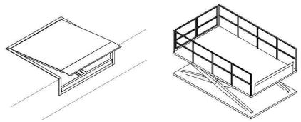
Depending on the configuration of the loading dock, Dock Levellers or Lift Tables can form part of the envelope of the building. Many suppliers offer insulated decking and/or air seals to reduce heat transfer.
